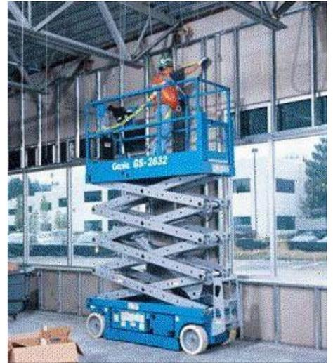
Planks, ladders or guardrail sides should not be used to gain extra reach or height. When working outside, mind the weather as wind can make a scissor lift unstable.
